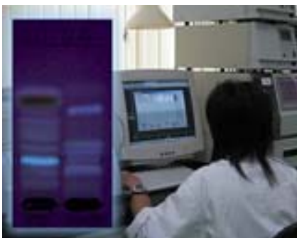
Thin Layer Chromatography (TLC) identifies the unique component make up of an herb while High Performance Liquid Chromatography (HPLC) ensures that the bio-active constituents are present in proper concentration
